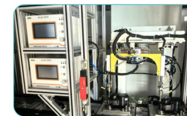
Air tightness test
