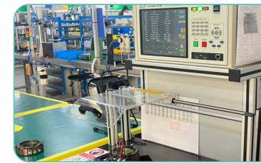
Stator Coil Inspection
