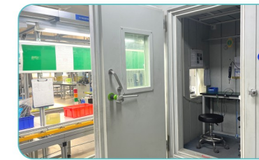
Motor assembly noise testing
